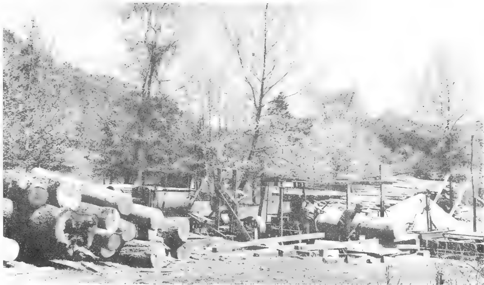
FIGURE 27.—This sawmill is typical of many small sawmills operating in Indiana. They usually set in or beside the woods and are generally operated by small gasoline or diesel engines.
