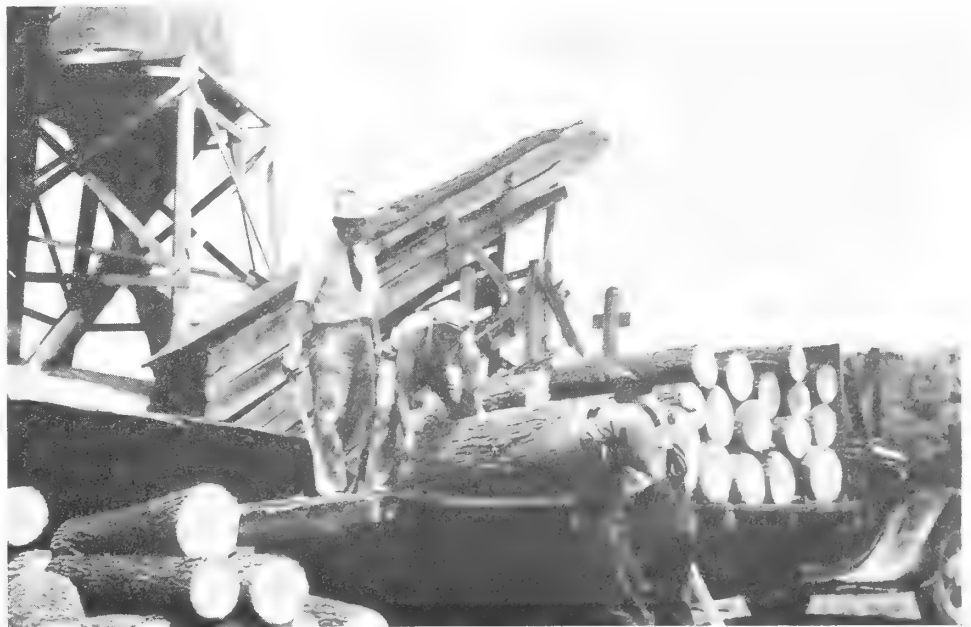
FIGURE 31.—Hickory bolts being delivered to an Indiana handle plant. Note the high percentage of white wood in most of the bolts—the wood preferred by the manufacturer.
