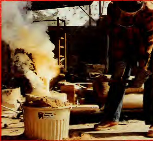
Dr. Ralph Staudt of the Art Department poses molten bronze into a casting mold. Photo from the Industrial Archive.
