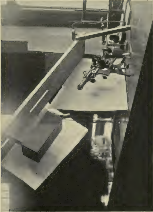
FIG. 2.—The photomicrographic apparatus. The microscope is ready to be used for direct observation. The gas-burner can just be seen at the lower end of the wooden plank. (N. B.—The sheets of white paper have been placed in this position in this and the next photograph in order to “showup” the apparatus.)
