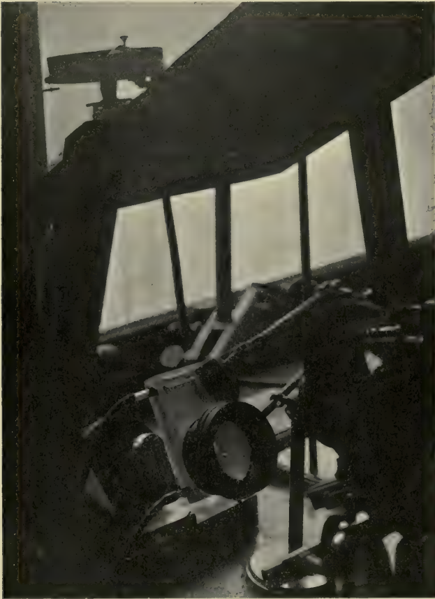
FIG. 5.—The photomicrographic apparatus. The microscope mirror is swung aside for photography.
