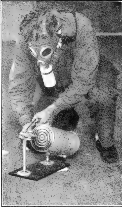
FIGURE 23.—Man, protected by gas mask, removing the top from a tin can containing discoids impregnated with liquid hydrocyanic acid.
