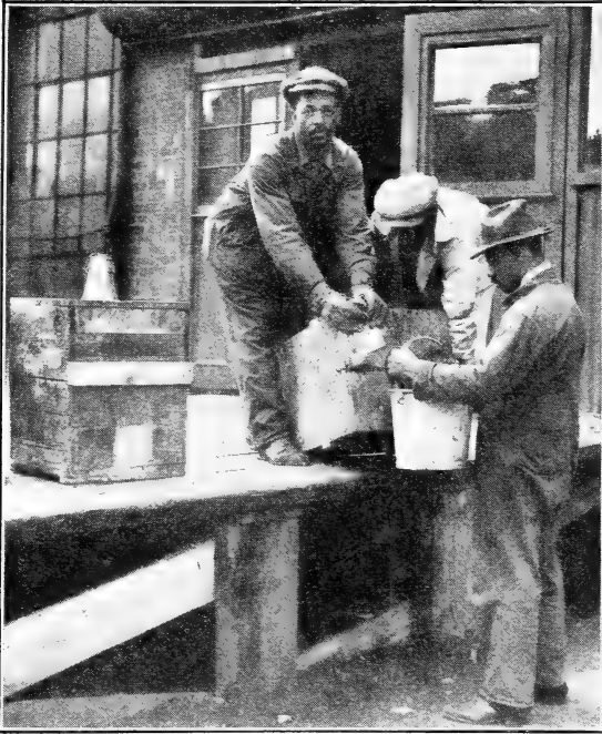
FIGURE 15.—A good illustration of workmen's indifference to spattering sulphuric acid. Most industrial plants have crews familiar with pouring acid; yet few are particular to avoid spattering and dropping acid.
