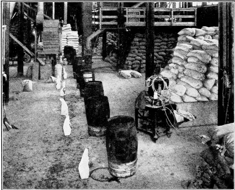
FIGURE 1.—Interior view in flour mill ready for fumigation with hydrocyanic acid gas generated by the barrel method. The eight barrels containing the acid-water mixture stand in galvanized-iron washtubs, and a sack of sodium cyanide is ready to be lowered into each barrel. Men lowering these sacks into the barrels, or working in any capacity around this or similar operations, should wear an approved gas mask and oiled leather gloves.
