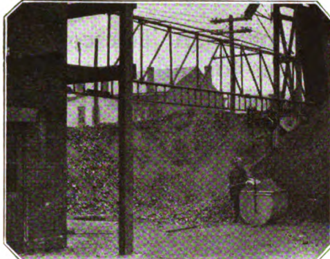
Handling coal on Louden Overhead Carrying System using a 36-foot Swinging Crane. Its 36-foot radius gives large coverage over coal pile. Handles loads up to one ton. Cranes built from 12 to 40 ft. in length.
