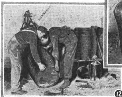
Figs. 11, 12, 13. What not to do. In the first place, don't drill out a hole in a good barrel; not only may the shavings contaminate the oil, but also you lessen the re-sale value of the barrel. Secondly, don't smoke in the oil room. Third, guard against spilled oil, for it is a fire hazard as well as being a hazard for you personally should you slip in it and perhaps injure yourself.
