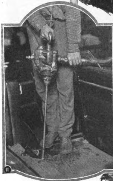
Fig. 11. Pneumatic tools operate under relatively low temperatures due to the expansion of the air in passing through them. Unless this air has been sufficiently preheated certain grades of lubricants may, therefore, be cooled to their points of congealment. It is, therefore, always advisable to select a low pour test oil. Naturally heavier tools will require heavier bodied oils; some are even built for grease lubrication.
