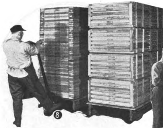
Fig. 8. The operator soon gets the knack of lifting the load by means of the truck handle.
