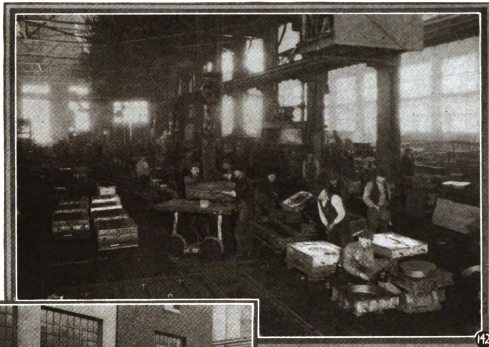
Fig. 142. On the jobbing foundry pouring floor, industrial railways and overhead traveling cranes are used on the majority of materials handling operations.
