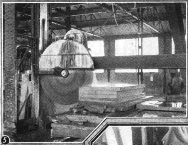
Fig. 5. Each 76 inch saw contains at least 100 black diamonds, and a sawing rate of an inch per minute is fast work.
