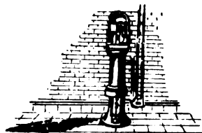
Feed Water Meter
