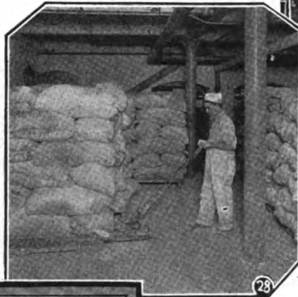
Fig. 28. Bags of flour in bakeries are now stored on platforms so as to eliminate unsanitary conditions and also to reduce handling costs.
