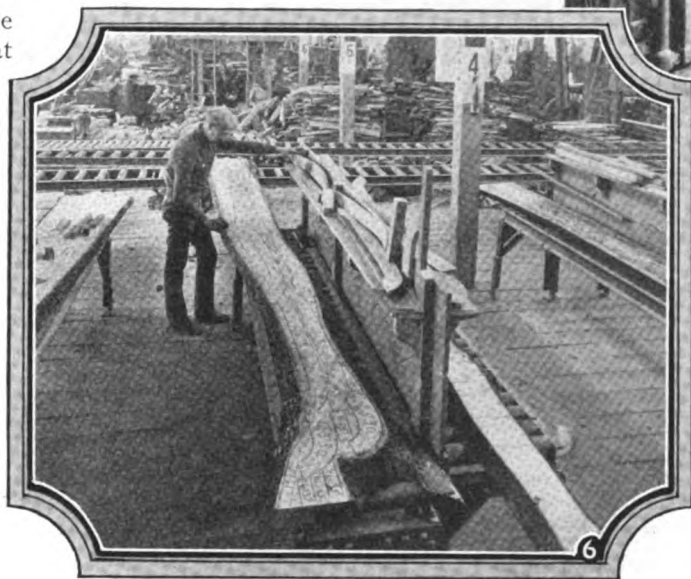
Fig. 6. The layout bench, where parts are marked off for sawing. Note how advantage is taken of natural curves in the plank.
