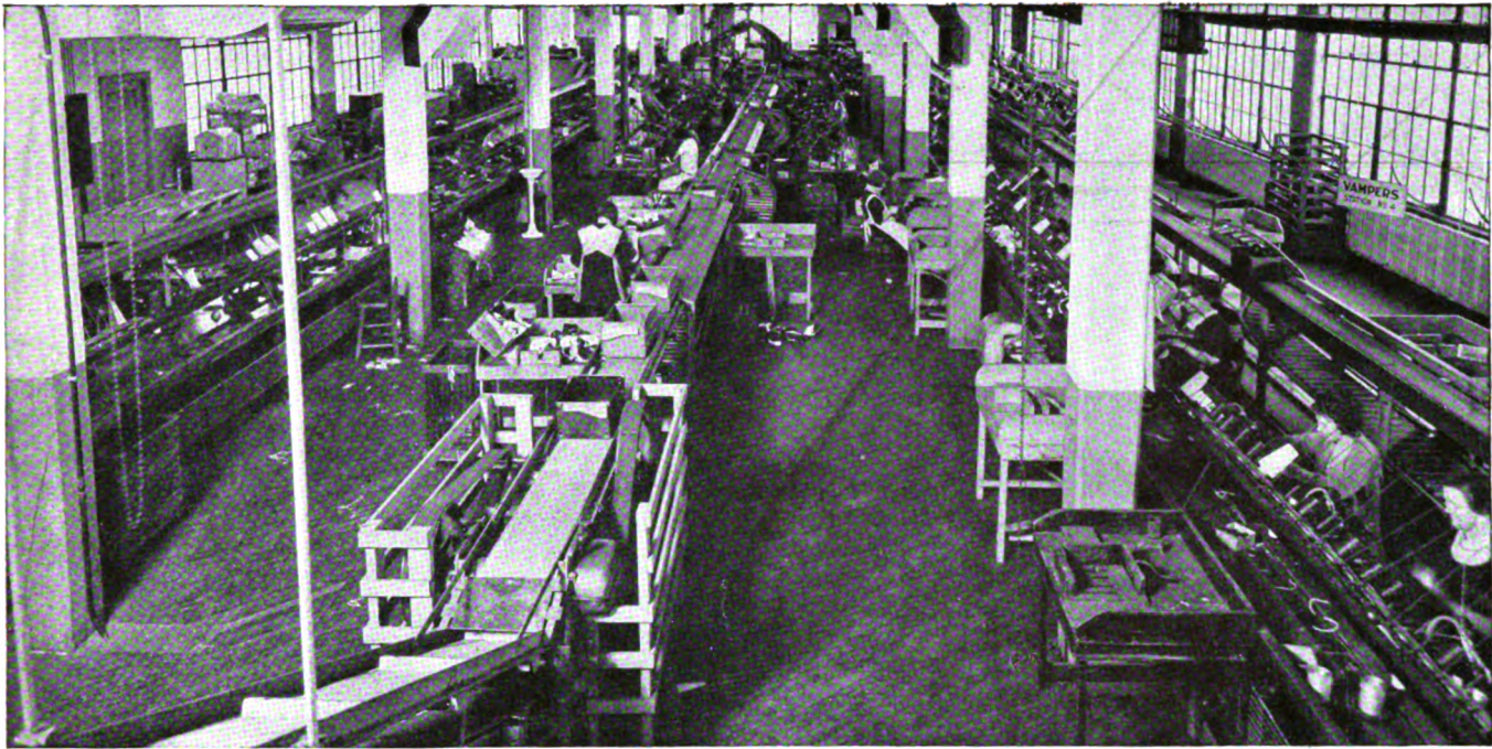
Materials are Lamson-conveyed through stitching room operations, illustrated above—Godman Shoe Co., Columbus, O.
