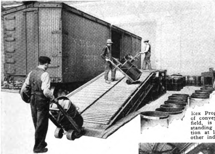
Rex Escalators (inclined loading conveyors) enable workmen to handle a great deal more tonnage with less fatigue and make possible a big saving in shipping costs.
