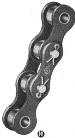
Fig. 14. Details of construction of a typical roller type of chain showing the connecting links, rollers, bushings and method of holding the pins in place by means of cotter pins.
