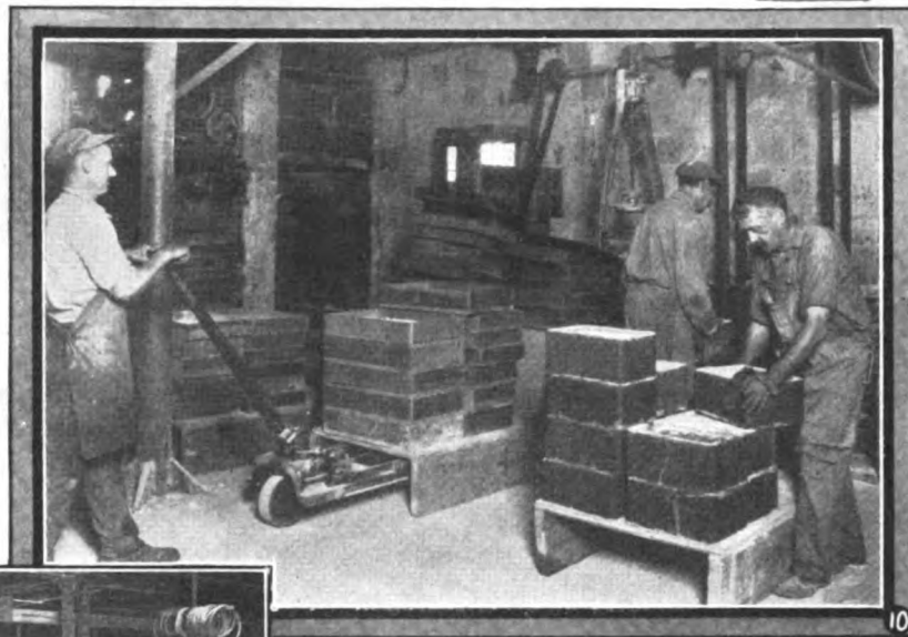
Fig. 12. Care should be taken in laying out aisles, as narrow aisles impede the operation of lift trucks.
