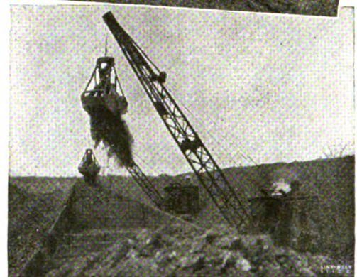
Upper—Link-Belt Power Hoe storing and reclaiming coal at the Electric Storage Battery Co., Philadelphia, Pa. (Mfrs. Exide Batteries). Lower—Link-Belt Locomotive Crane loading and unloading coal in storage.
