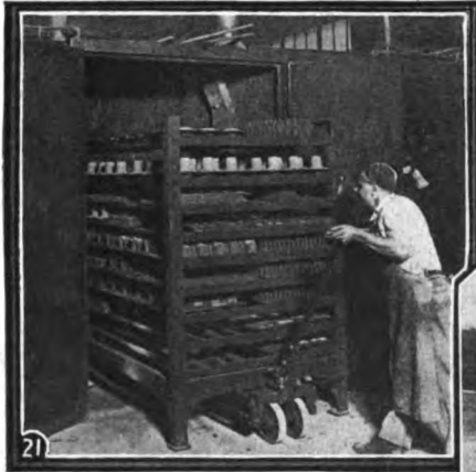
Fig. 21. For handling fragile materials, lift trucks are now equipped with springs which absorb shock in transportoin.
