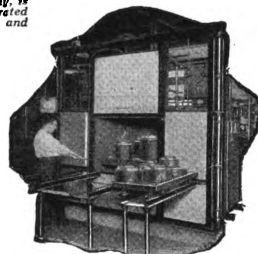
Baking, drying, and other oven processes are improved by the utilization of electric heat. G-E heating equipment with automatic control is used most extensively in this field.
