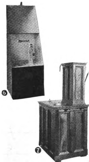
Figs. 6 and 7. Two types of cabinet oil storage tank which are not only serviceable but also efficient. Individual storage tanks are extensively used in many plants where it is not absolutely necessary to go to the expense of installing an extensive oil house layout. Especially is this true where but a few grades of oils are used, and these in but small quantities.
