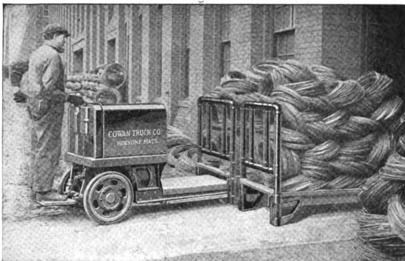
Photograph shows Cowan Electric Lift Truck picking up "skidded" load of coils of wire in plant of Geo. W. Prentiss & Co., Holyoke, Mass.
