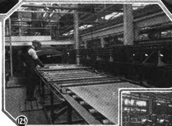
Fig. 125. The discharge from the lehr is clearly visible and the man is cutting the glass into the desired length.
