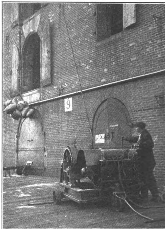
Fig. 23. Portable hoisting units should have all the machinery carefully guarded to keep foreign materials from falling into the moving parts.
