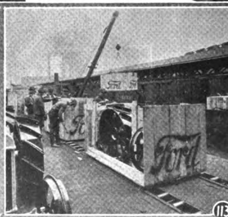
Fig. 113. Fordson tractors being packed for export and loaded direct to flat cars. Note the gravity conveyors in the floor that assist in moving the heavy cases.
