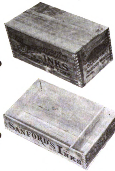
Figs. 16 and 17. The locked-corner box, of comparatively light wood, as used for the shipment of bottled inks.
