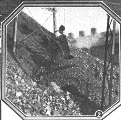
Fig. 2. Discharging of coal from a bucket operating on a monorail cable storage system.
