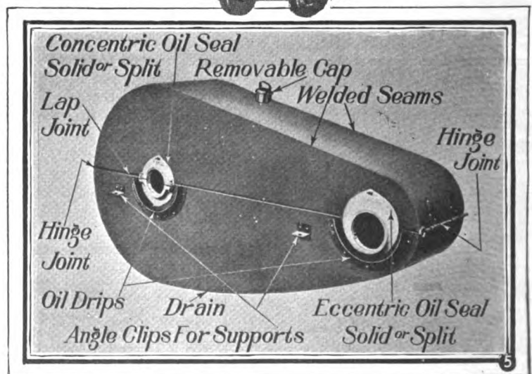
Fig. 5. An oil retaining silent chain casing. The essential details of constructions are clearly shown by the respective notations.
