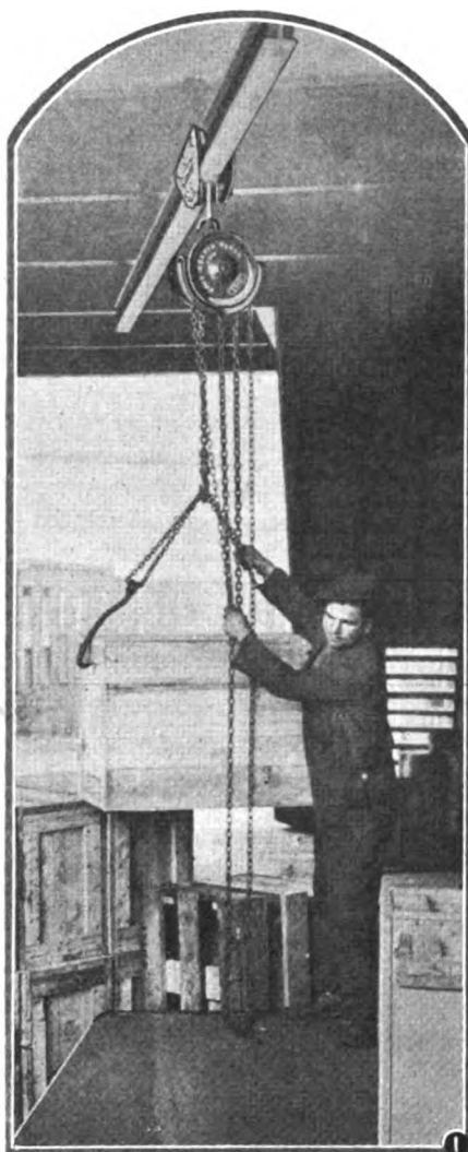
Fig. 1. A good pair of tongs and a piece of strong chain make an excellent combination for the speedy handling of a variety of bulky loads.
