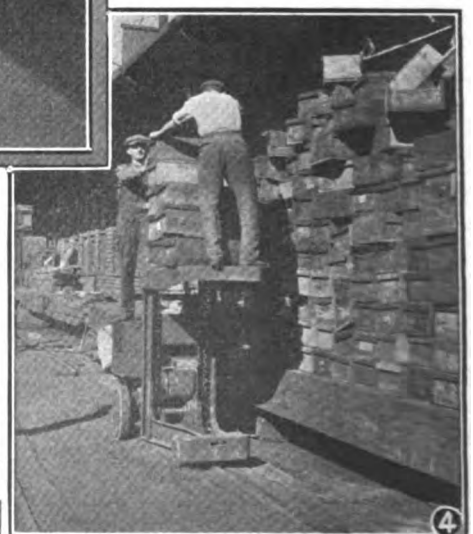
Fig. 4. Operating industrial trucks over rough ground and sharp railroad tracks is both dangerous and expensive.
