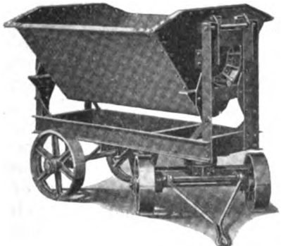
A one yard "V" dump body may be mounted on the fifth wheel trailer for handling loose materials.
