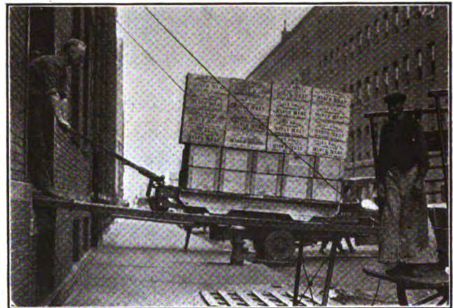
Fig. 34. Note the brake on the front wheels to hold the load on the incline.
