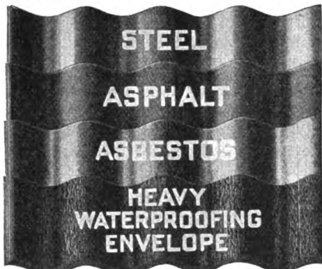
Cut-away View of a Small Section of Asbestos Protected Metal
