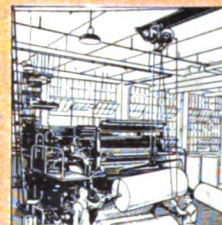
Loading heavy bulky paper rolls onto presses with a LiftAbout.
