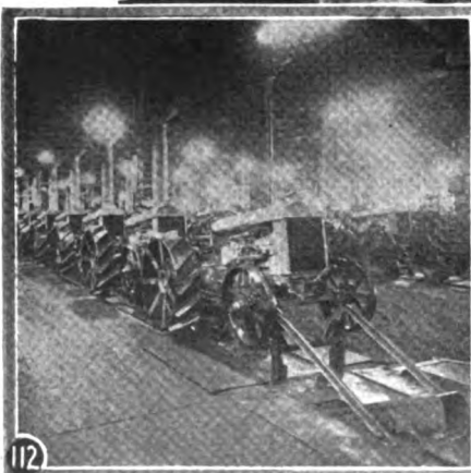
Fig. 112. Discharge end of the tractor assembly conveyor showing Fordson tractors completely assembled.
