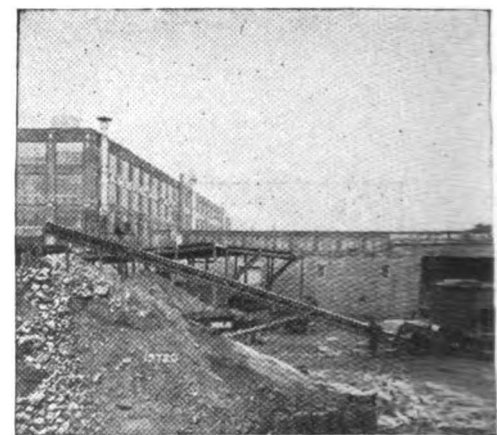
Portable Car Unloader—Loads coal from hopper-bottom cars to storage or truck, at low cost, saving demurrage charges.
