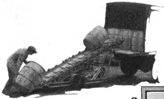
Fig. 6. Portable slat conveyors of this type stand a lot of abuse but frequent alignment and good maintenance will increase their life.
