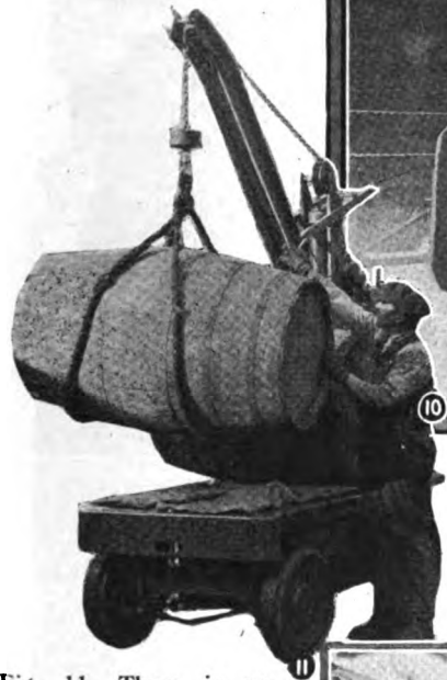
Fig. 11. There is no danger of dropping a barrel hung in this fashion so long as the sling is properly tightened about each end of the barrel.
