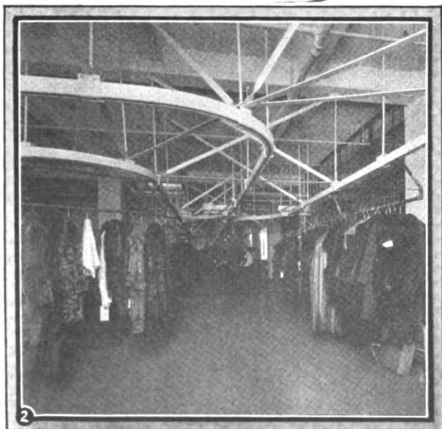
Fig. 2. General view of the receiving and shipping room showing overhead carrier system or method of transporting the pieces or garments into and out of storage.
