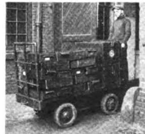
This junior member of the group carries a 3000-pound load down a three-foot aisle.
