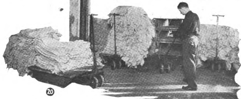
Fig. 20. Production material of an unwieldy nature should be piled on platforms and only re-handled when required for production purposes.
