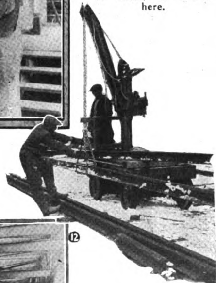
Fig. 12. In loading rails on the electric industrial truck shown here, note the block of wood used to keep the strands of the sling chain apart so that the rail is properly balanced.
