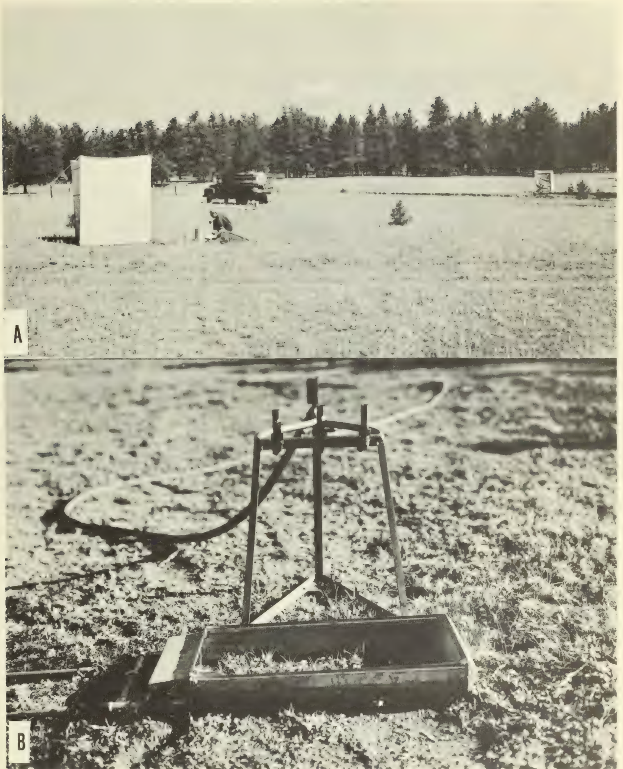
Figure 8.-- A , Rocky Mountain infiltrometer during the field operation in grassland; B , Closeup of rainfall applicator, rainfall troughs, and runoff plot which are enclosed by tarpaulin windbreaks during field tests.
