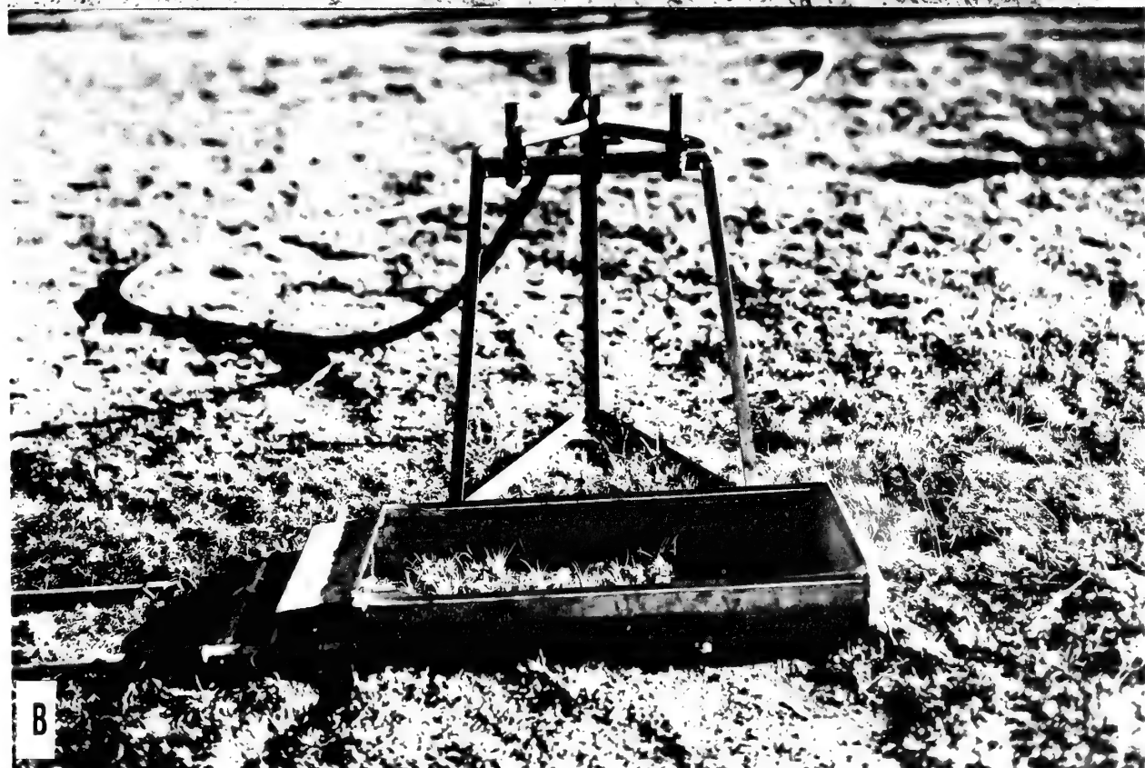
Figure 8. -- A , Rocky Mountain infiltrometer during the field operation in grassland; B , Closeup of rainfall applicator, rainfall troughs, and runoff plot which are enclosed by tarpaulin windbreaks during field tests.
