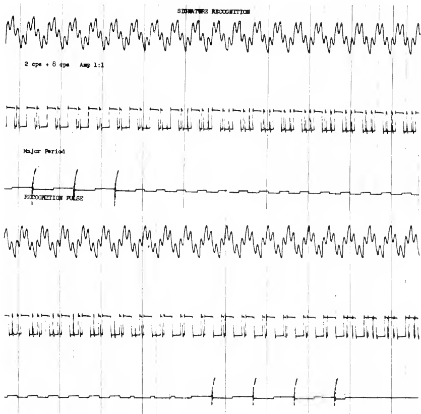
Fig. 11. Recognition of a "fat-thin-fat" Square Wave Set. The synthetic function of mixed sine waves slowly changes wave shape over time. If, and only if, the wave shape generates a square wave sequence within acceptable limits, the complex is "recognized," as indicated by the spike in the recognition pulse trace.
