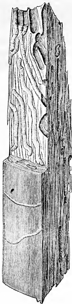
FIG. 26.—Work of the banded ash borer ( Neoclytus caprea ). Section of ash log showing larval mines. (Original.)
