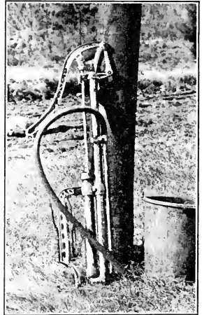
FIG. 57.—A bucket pump. Original.
