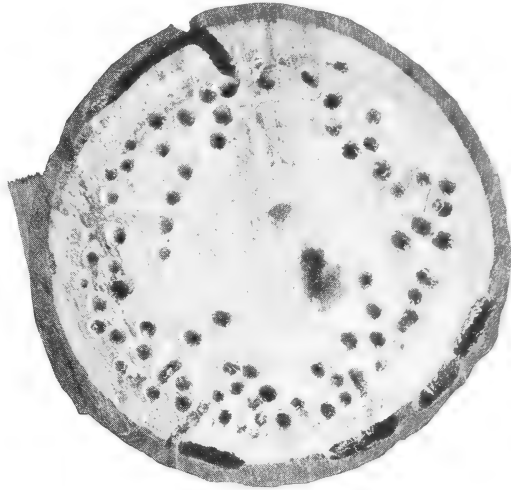
FIGURE 49.—Cross section of persimmon low showing the wood destroyed by grubs of the powder-post beetle Xylobiops basilaris . (Natural size.)
