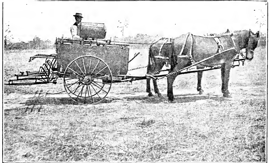
FIG. 225. — Fieldsprayer, with modifications, adapted for potato spraying by L. C. Corbett, operating at the Virginia Truck Experiment Station, Norfolk, Va. 263
