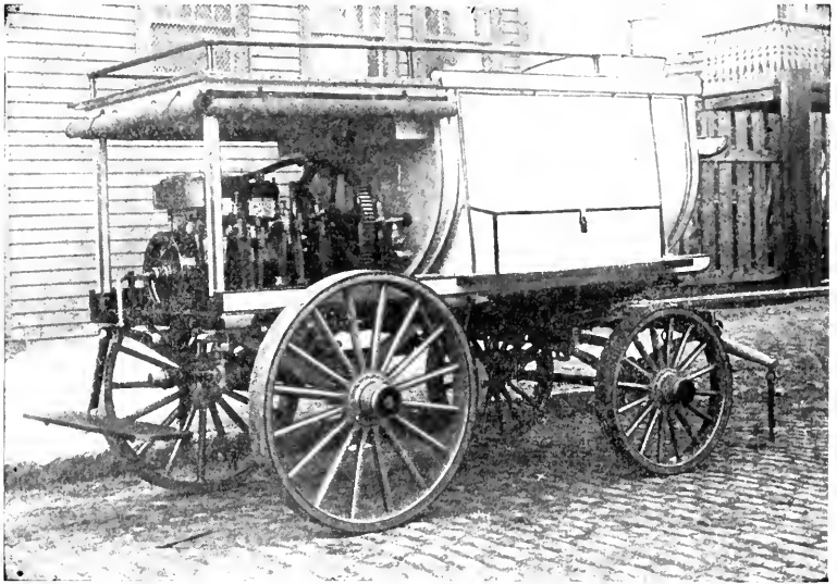
FIG. 38.—One of the latest three-cylinder power pumps designed for spraying shade-trees and woodlands.
