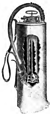
FIG. 32.—Compressed-air sprayer with section of tank removed to show air pump within.
