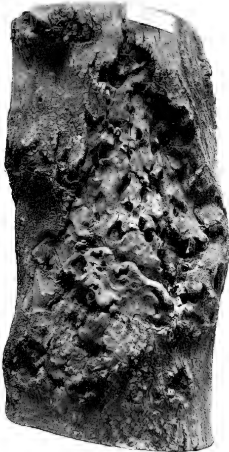
Work of carpenter worm in ash
