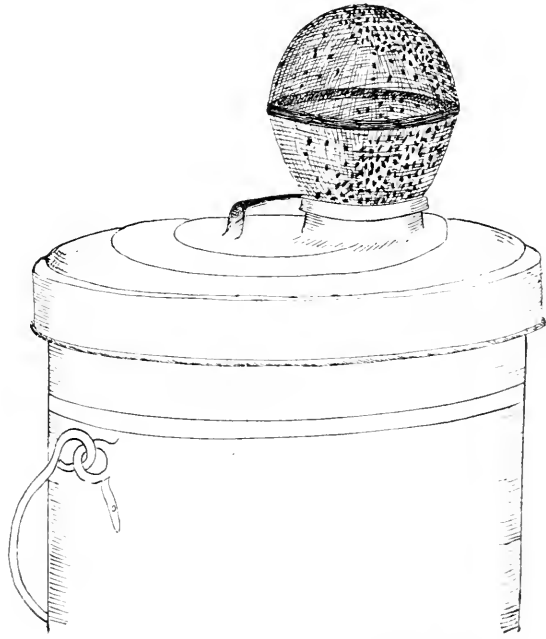
FIG. 8. — Hodge's trap for garbage can.
