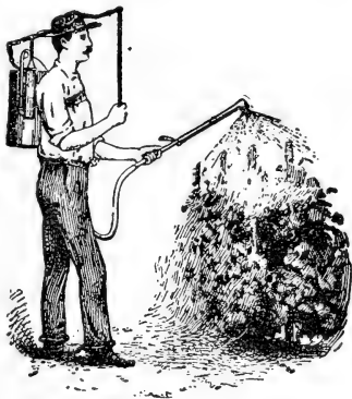
FIG. 18. THE KNAPSACK SPRAYER.
