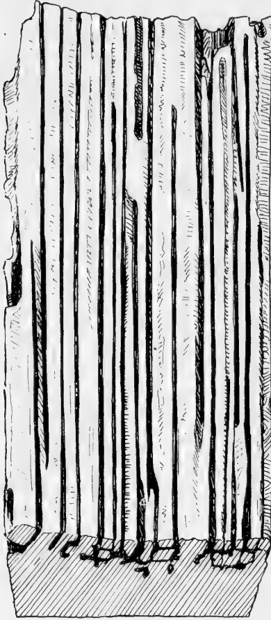
FIG. 76. Termite work in a piece of wood. Tunnels following the grain are made by species of Reticulitermes , the common underground termites of the eastern United States
