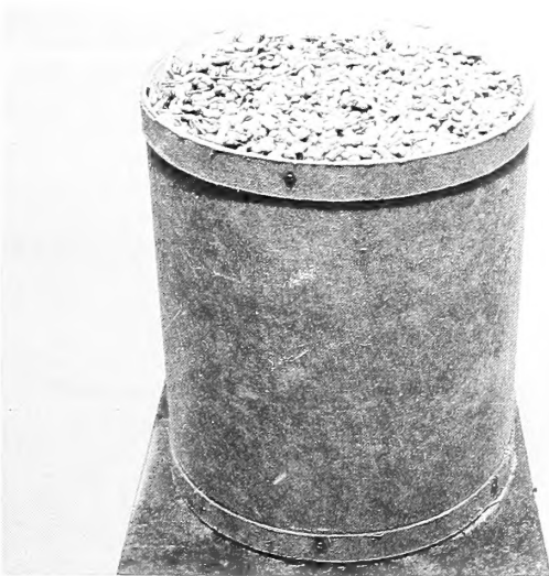
Figure 1. --Five-cubic-foot masonite bin filled with peanuts exposed to vigorous infestation of stored-product insects.
