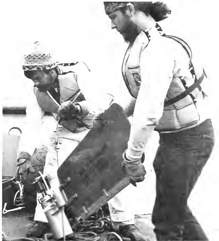
Dale Pillsbury and Ben Moore ready a CUE-I Aanderra current meter that will be suspended beneath the OSU buoy.
