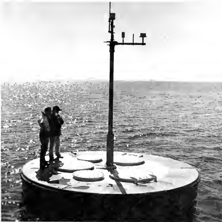
The SODS buoy measures thermocline oscillations and an apparent bottom mixed layer during CUE-I.
