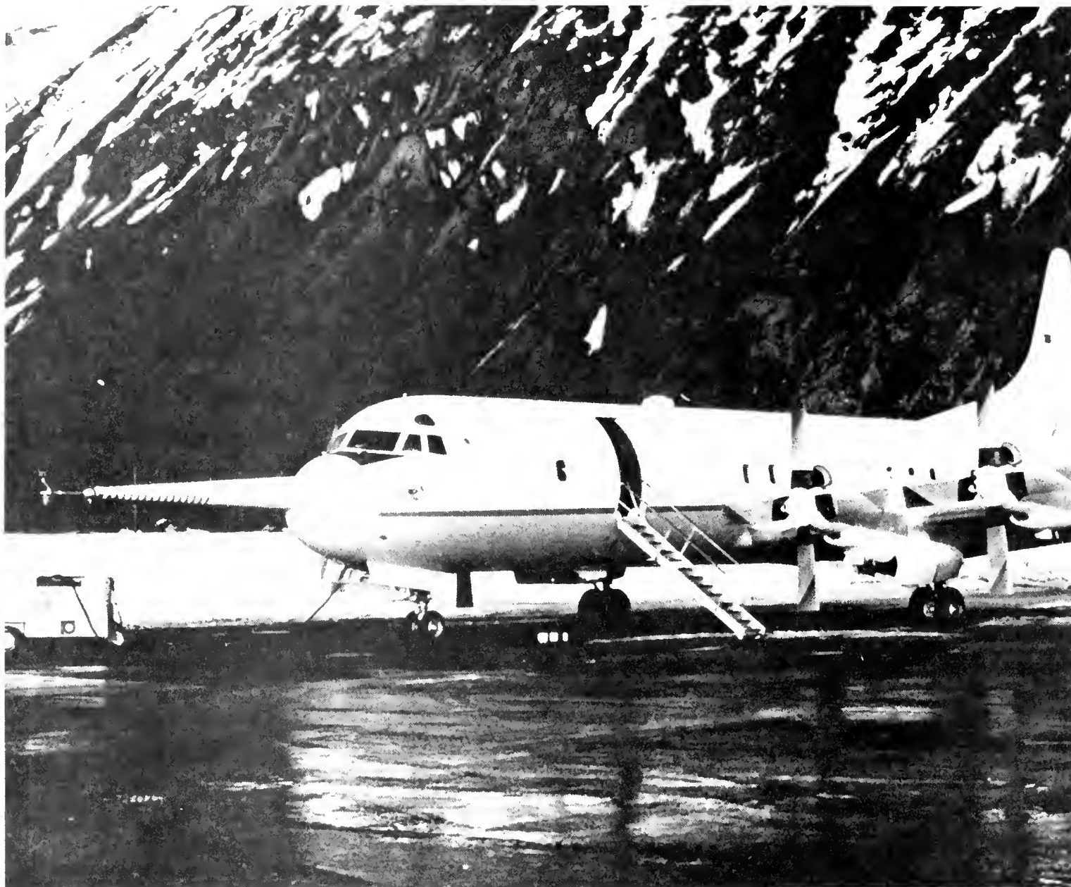
NCAR Electra at Kodiak, Alaska, March 1975. NORPAX flights over ocean in regimes of high wind speed directly measure air-sea flux of heat, momentum, and moisture by means of instruments mounted on nose boom.
