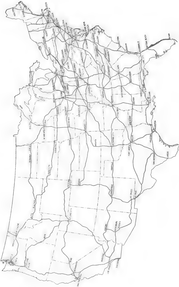
FIGURE 1.—The general location of routes of the recommended interregional highway system. Total length of the system is 33,920 miles.
