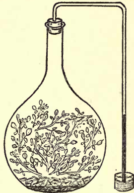
FIG. 82.—APPARATUS TO SHOW THE ABSORPTION OF OXYGEN BY A GREEN PLANT.
