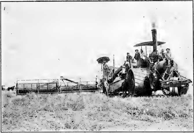
A 50-HORSE-POWER COMBINED STEEL HARVESTING MACHINE AND THRESHER. (Steam power.) Front view, showing the wheat being cut.
