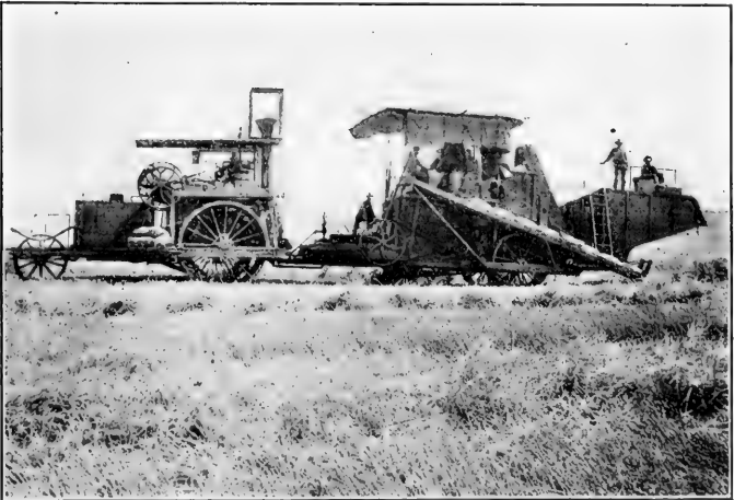
COMBINED HARVESTER MACHINE. Side view. The machine cuts the wheat, threshes it, and delivers it ready sacked in one continuous operation.
