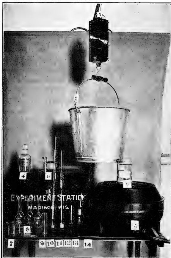
BABCOCK TEST OUTFIT. 1, spring balance for weighing milk; 2, milk pail; 3, galvanized-iron box for keeping samples of milk; 4, sulphuric acid; 5, Babcock hand tester; 6, composite sample jar; 7, beaker for adding acid; 8, Babcock test bottles; 9, acid measure; 10, 25-c.c. pipette; 11, 17.6-c.c. pipette; 12, clinical thermometer; 13, hydrometer for determining strength of sulphuric acid; 14, note-book.
