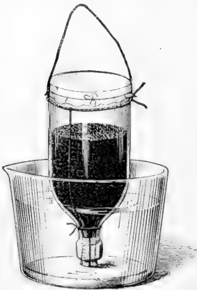
EXPERIMENT SHOWING ABSORPTION OF WATER BY SOILS.
