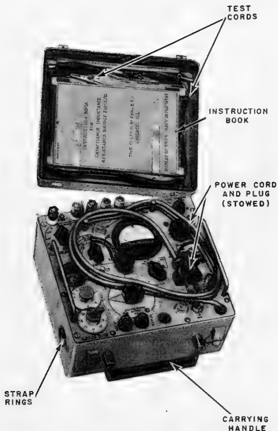
20.345 Figure 10-15.—Capacitance-inductance-resistance bridge, type ZM-11/U.
