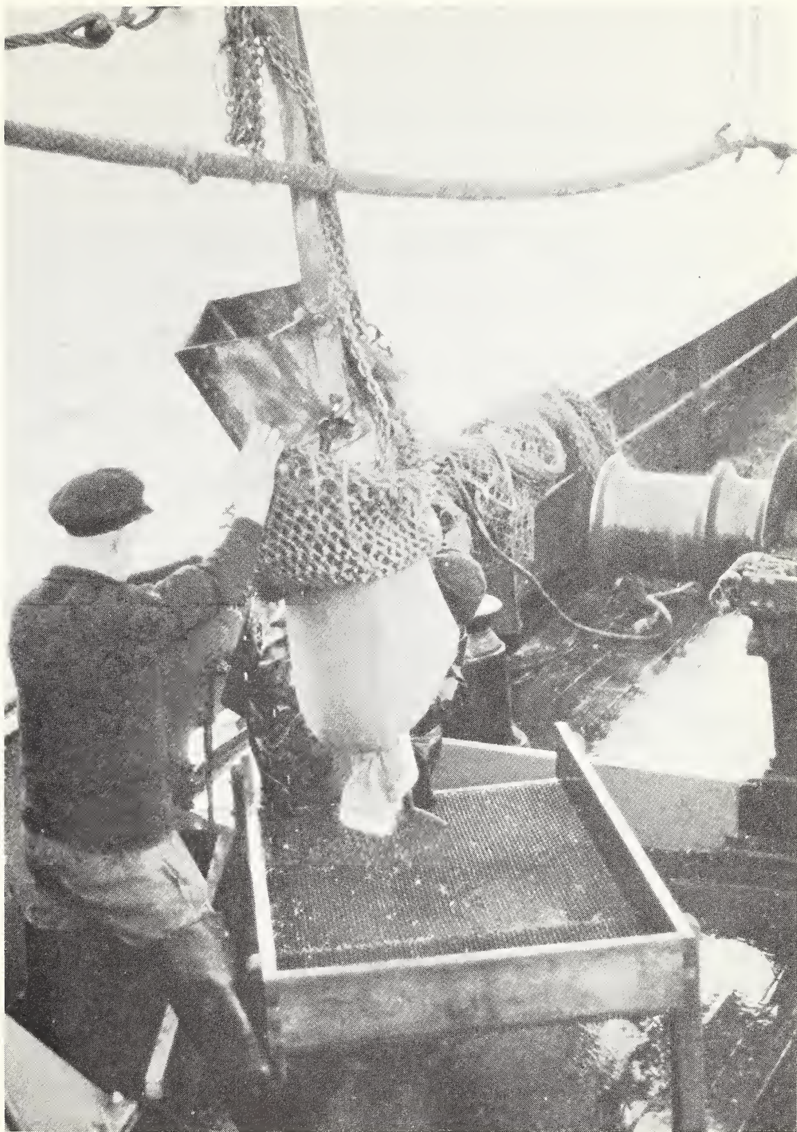
Plate 15 Anchor dredge about to be emptied on-board ship
