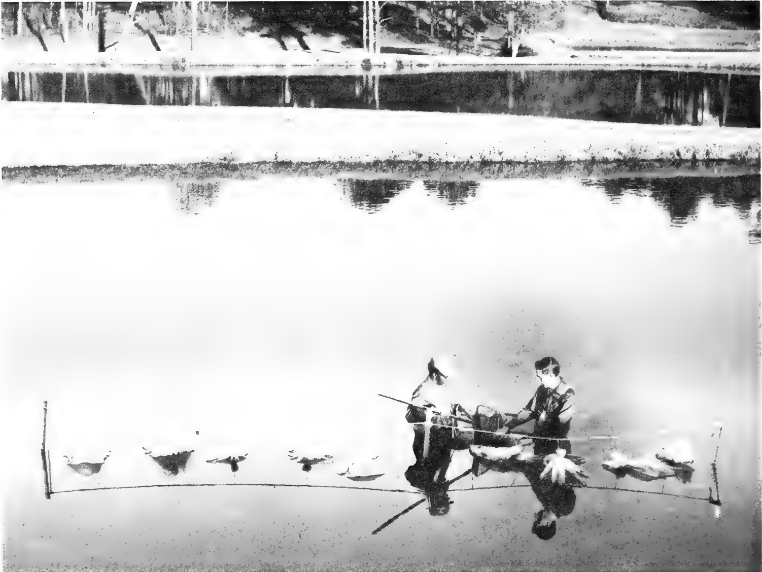
Figure 1. Sample apparatus for suspending large plastic bags used to conduct on-site toxicity tests.
