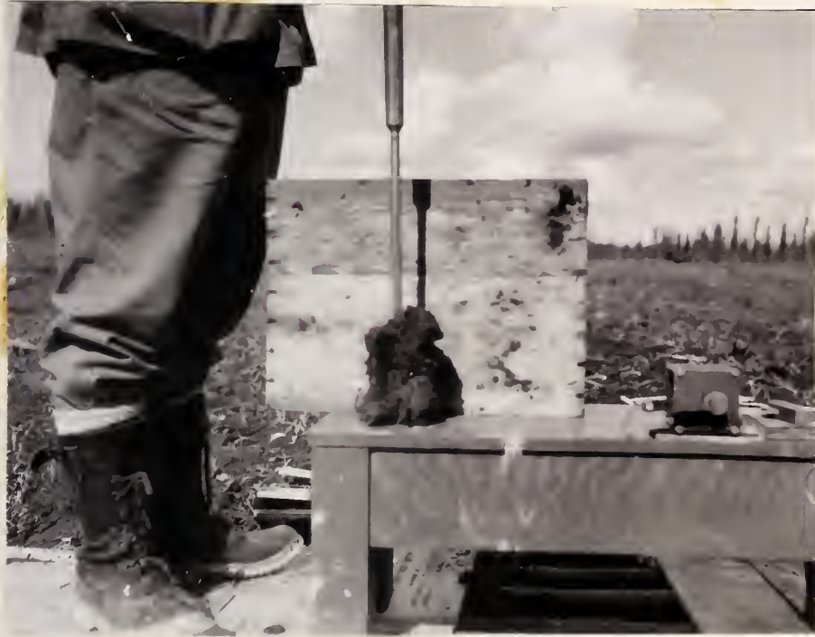
Fig. 14 Muskeg soil adhering to the vanes of the apparatus
