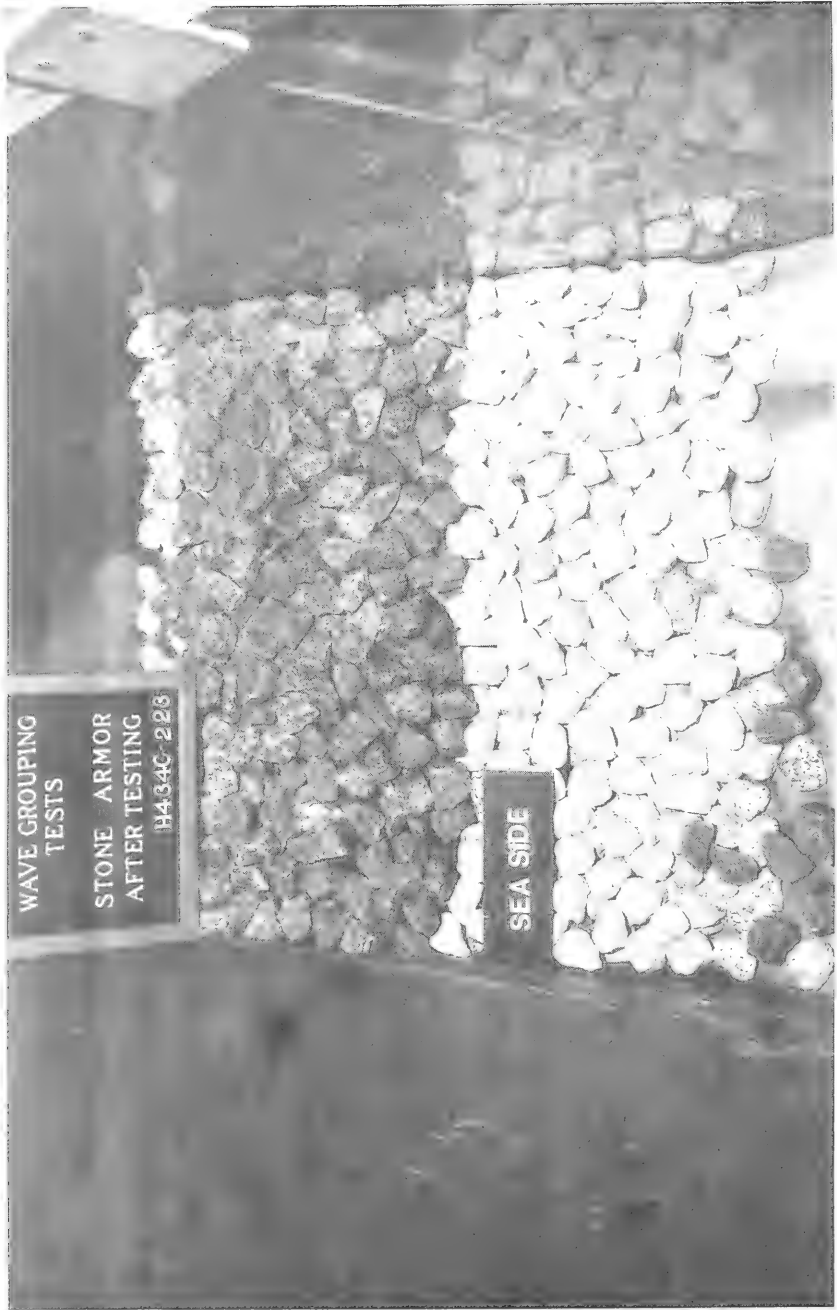
Photo 8. Sea-side view after wave attack of 4.0-sec, 0.30-ft waves at the 0.80-ft depth; \gamma = 20
