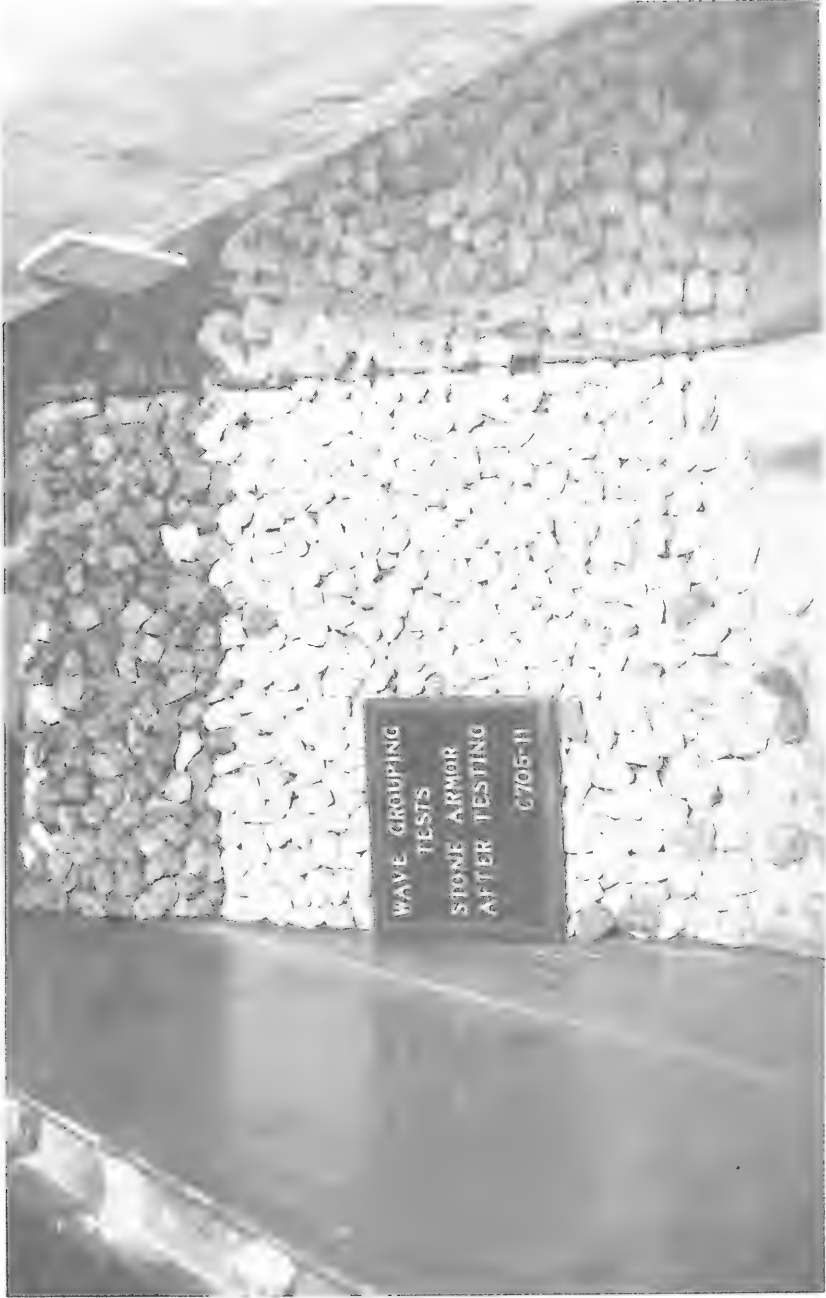
Photo 11. Sea-side view after wave attack of 2.25-sec, 0.36-ft waves at the 1.60-ft depth; gamma = 20
