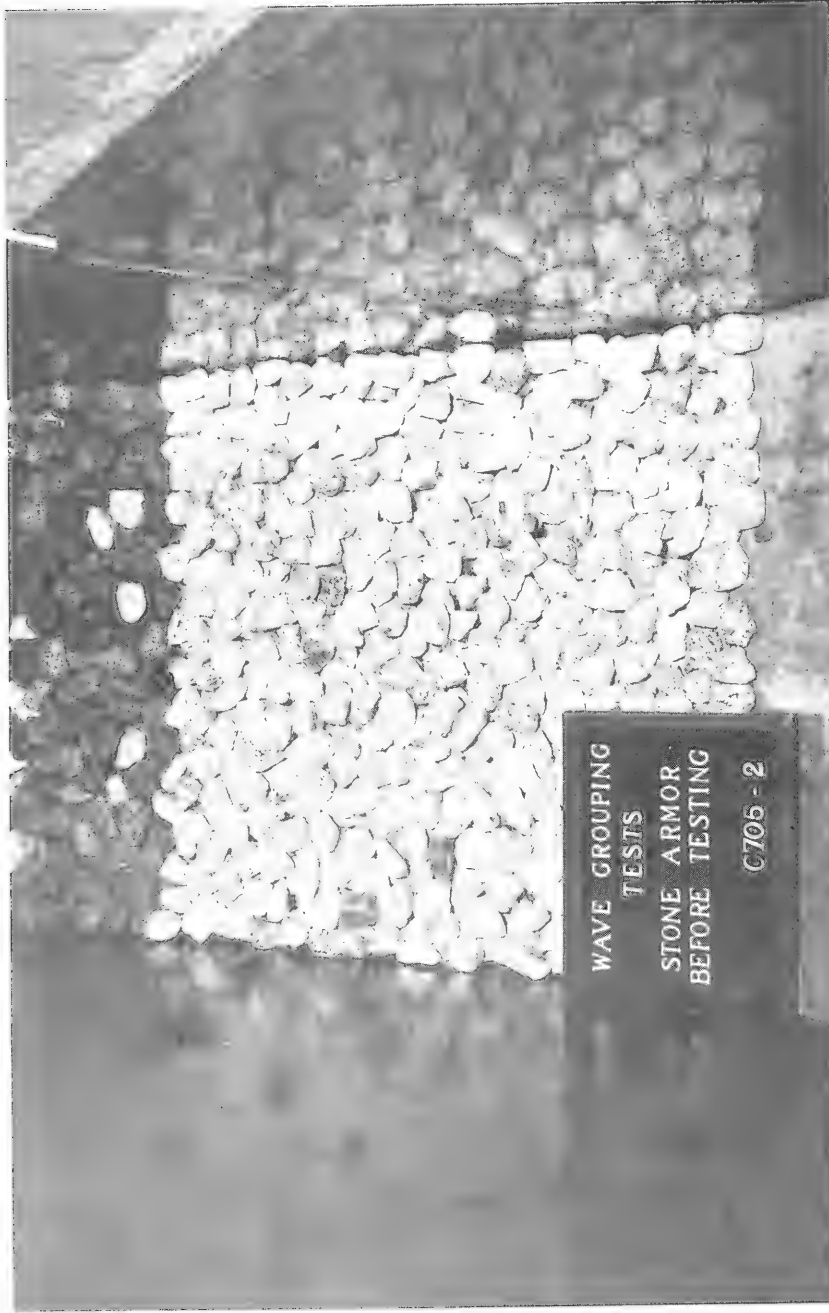
Photo 4. Sea-side view before wave attack at the 1.60-ft depth. Change in stone color denotes still-water level
