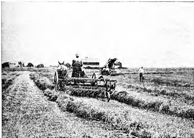
Courtesy International Harvester Company. Fig. 28.—The side delivery rake is considered the most important implement in the economical making of alfalfa hay of good quality on a large scale.
