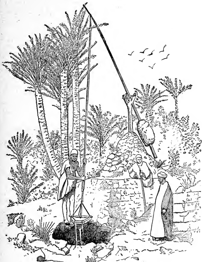
Fig. 80. Shadoof of Egypt, or Paecottah of India. (Wilson, U. S. Geol. Survey.)
