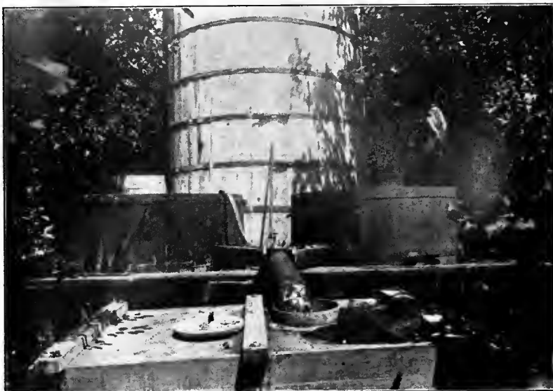
Fig. 5. Mixing apparatus, showing method of combining the streams from dilution tanks before they enter the sprayer.
