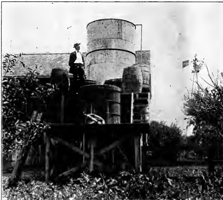
Fig. 4. A convenient type of mixing apparatus, showing stock solution barrels, dilution tanks, and elevated water power.
