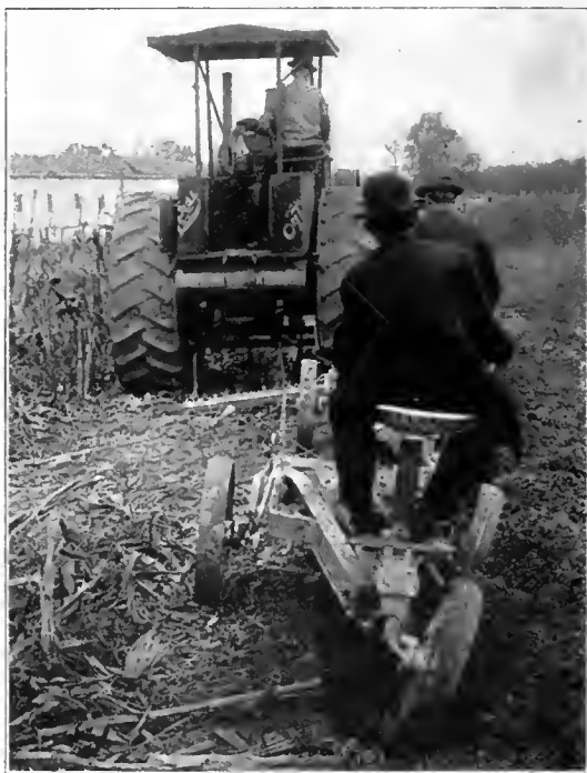
Rumely Oil-Pull Tractor (15-30 h. p.), Pulling Two Spalding Deep Tilling Machines, 10 to 15 Inches Deep. Engine Had Sufficient Power to Haul Another Machine.
