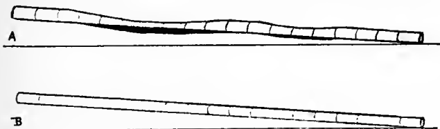
A Shows Improper Grading and Laying of Tile. B Shows Proper Grading and Laying of Tile.
