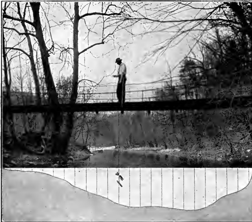
Plate I.A. Showing Method of Measuring Cross Section of River.
