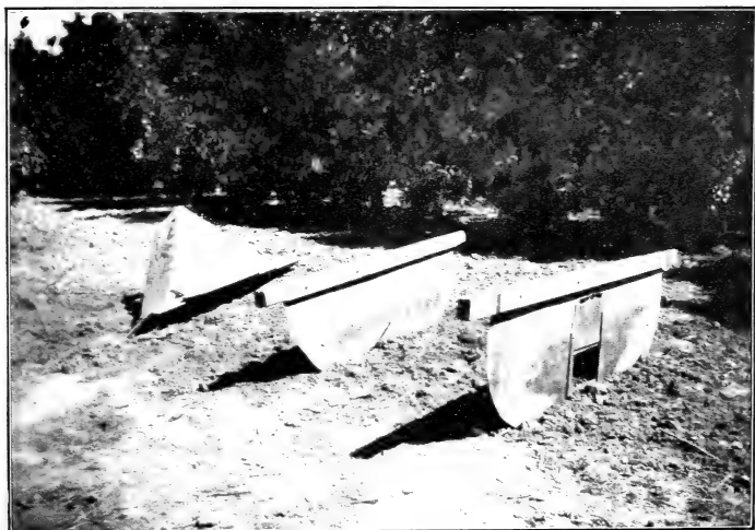
FIG. 2.—THE V-SHAPED "CROWDER" AND METAL DAMS OR "TAPPOONS."
