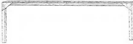
FIG. 7.—Handy level for locating large furrows in hillside irrigation.
