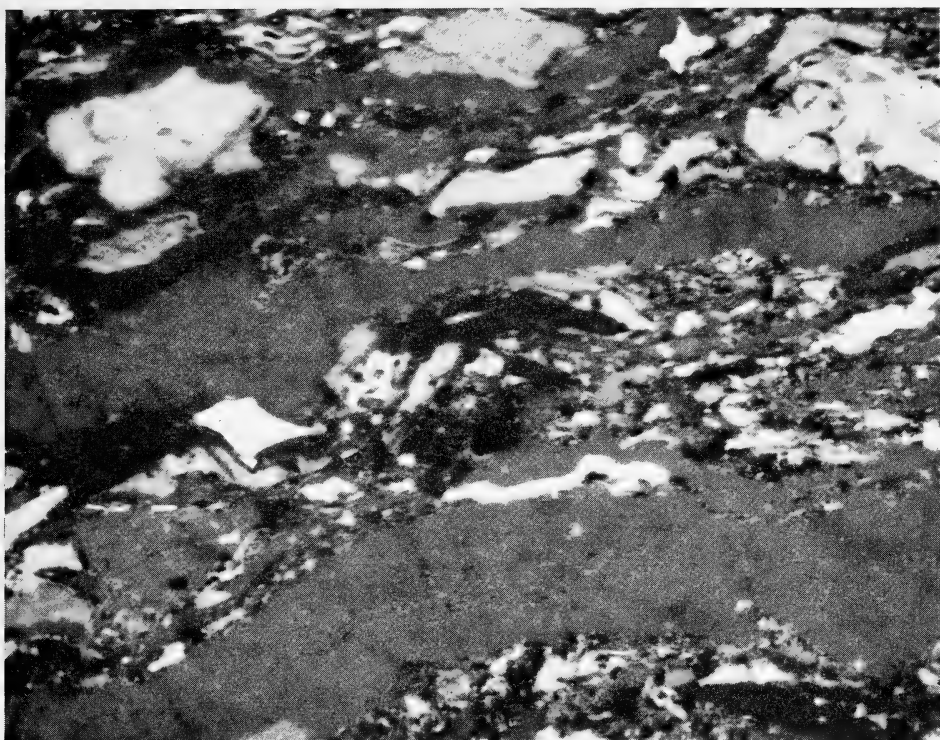
FIG. 3 Thin layers of vitrinite, grey, with micrinite, light grey to white and exinite dark grey. Reflected light, oil immersion. 700 \times .
