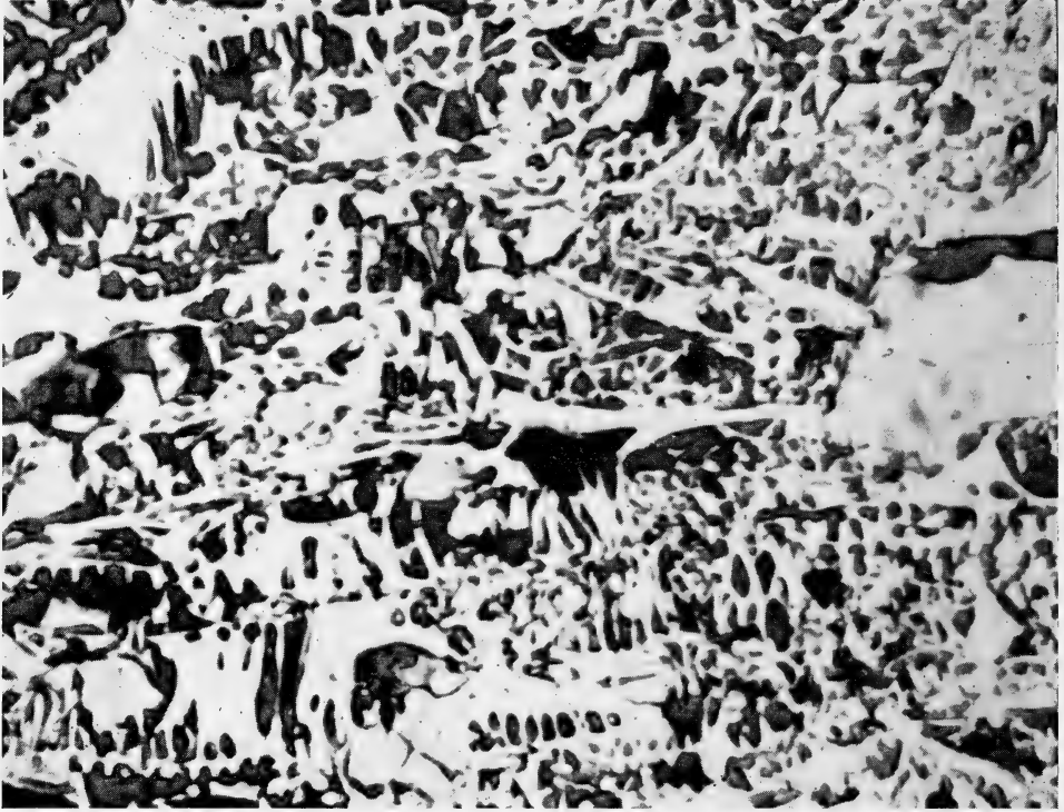
FIG. 4 Semifusinite showing scalariform pitting. Cell lumens filled with material of vitrinite reflectance. Reflected light, oil immersion. 700 \times .
