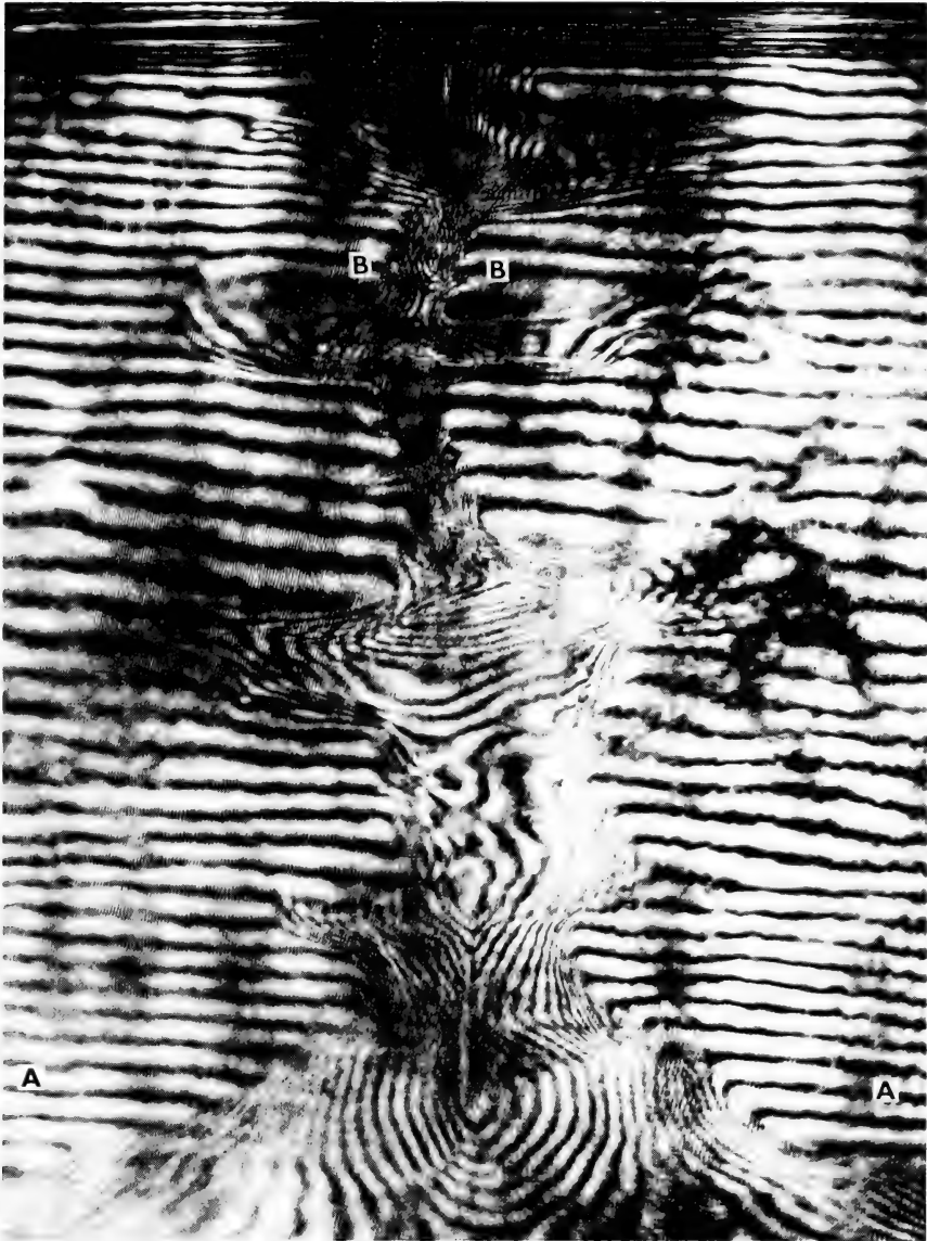
Figure 4. Interferogram of a pinched discharge in a plasma focus geometry. The length of the discharge shown is 3 cm. The discharge current is 0.85 MA, n_e \sim 5 \times 10^{19} \text{cm}^{-3} , T_e \sim 2 \text{keV} , exposure time 1.2 \times 10^{-9} \text{s} .
