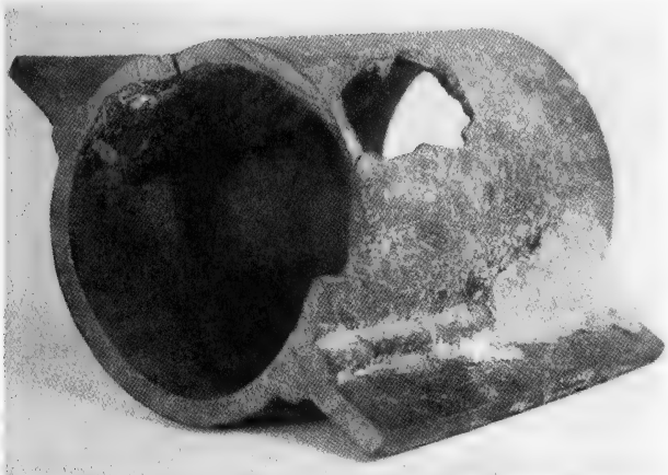
Fig. 1. Cut length of a high-pressure boiler tube corroded from the inside (the waterside), showing thick-edged hole about 4 cm long where steel embrittled by hydrogen (corrosion by-product) was violently ejected while boiler was operating.
