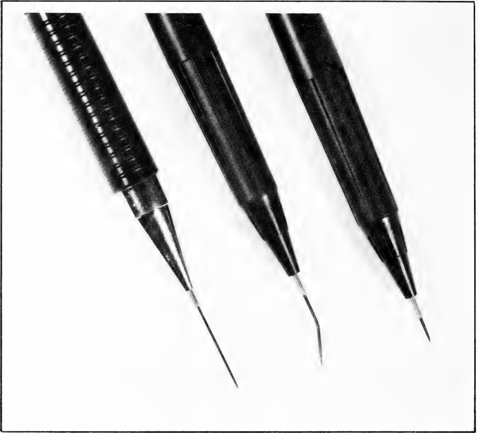
FIG. 1. Heads of three mechanical pencils with lead replaced by Nos. 1 (left) and 4 (middle and right) entomological pins. Left hand probe adjusted for long working length.
