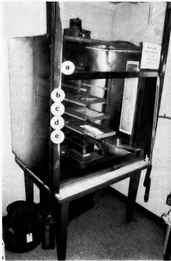
Fig. 2. Fumigation apparatus in fume hood for surface-sterilizing codling moth eggs with formaldehyde fumes: (a) exhaust fan, (b) empty tray, (c) tray with egg-laden waxed paper, (d) tray with egg-laden polystyrene pellets, (e) stainless-steel container for formaldehyde.
