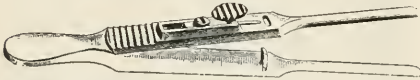
Fig. 2. Ehrlich's cover-glass forceps, for holding cover-glasses for securing thin film of blood.
