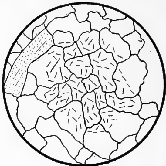
FIG. 1.—Quartz Mosaic, with hair-like inclusions, from Rowlandville granite. x 80.
