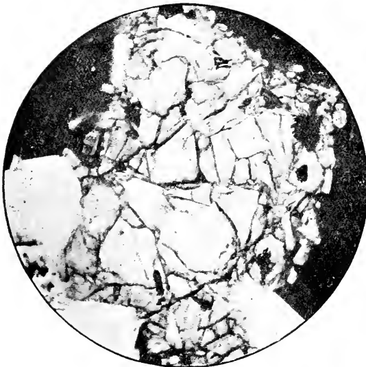
Fig. 39.—Cracked olivine core with a rim of hypersthene crystals in the land-lava of the western field.
