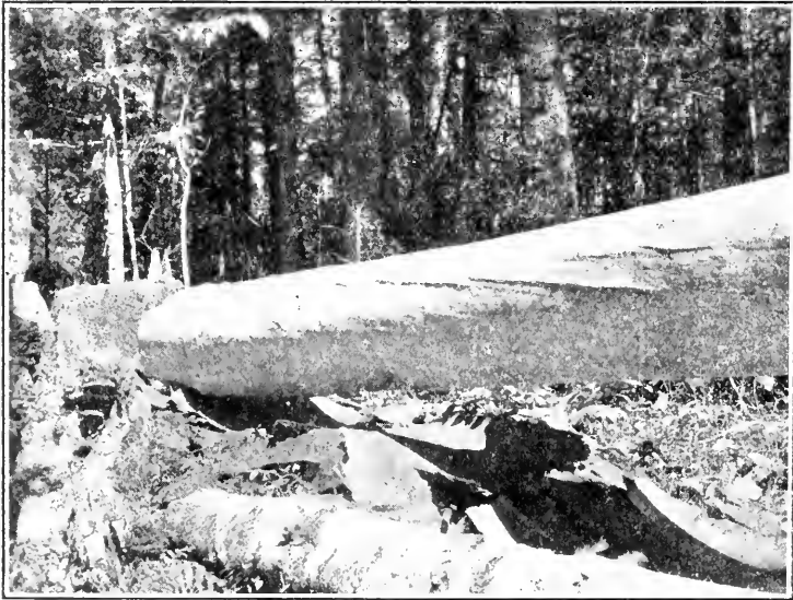
Red spruce large enough to cut clear lumber but spoiled for airplane use by spiral and pitch seams
