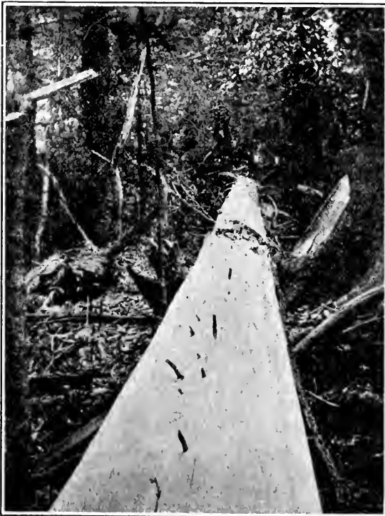
Straight-grained clear spruce tree split in falling, showing prevalence of knots in the heart of all red spruce. The grain of the heart spirals to the left.
