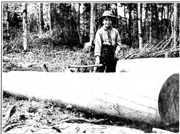
Spruce log showing severe right spiral and deep season-checks from removal of bark. Log cut a month previous for pulp.
