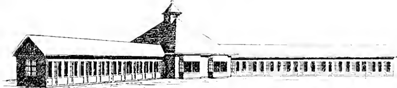
Fig. 29. Elevation of part of a sanatorium pavilion of Doecker construction for 20 beds. The administration buildings are not shown
