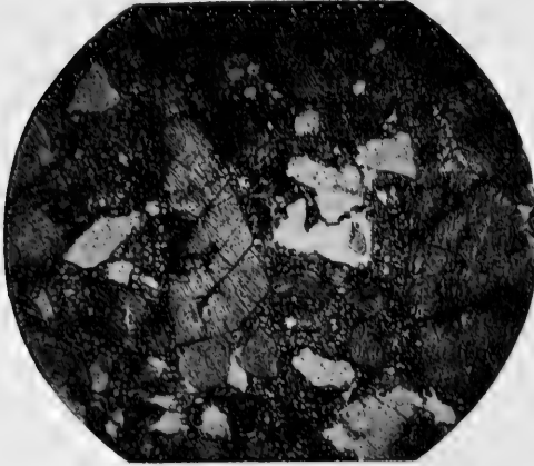
FIG. 4.—Photomicrograph of Pondville (Mass.) arkose, an arkose formed under moist temperate conditions, showing the quartz and feldspar grains in a fine-grained matrix of quartz and argillaceous material. Magnification, 15 diameters.
