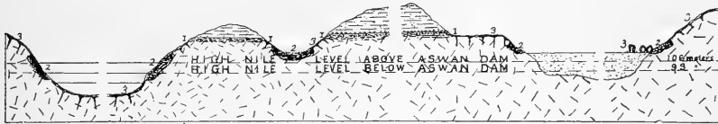
FIG. 1.—Diagrammatic section across the region of the Aswan Cataract. 1, Disintegrated and decomposed zone at the base of the Nubian Sandstone. 2, The massive granular disintegration. 3, Disintegration of the present.
