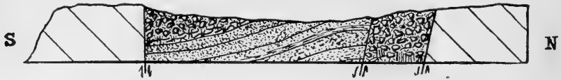
FIG. 16.—Structure section, G, through Clarke's Head, on the south, and Swan Creek, on the north. The structure of the pre-Triassic rocks is not shown. Overlying the Triassic red sandstone is a bed of tuff, overlain, in turn, by agglomerate. At Swan Creek only agglomerate appears, but it is probably a part of the same flow.
