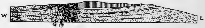
FIG. 22.—The shore section along Gerrish Mountain, as seen from the eastern end of Moose Island. The Triassic sandstone, at the left, is faulted against a mass of agglomerate overlain by a capping of sandstone. The agglomerate is probably faulted against the dike of diabase, which has fed the basalt flow which caps the cliffs on the right. At the base of this flow is a bed of green ash, and beneath this is normal Triassic sandstone, with some shale.
