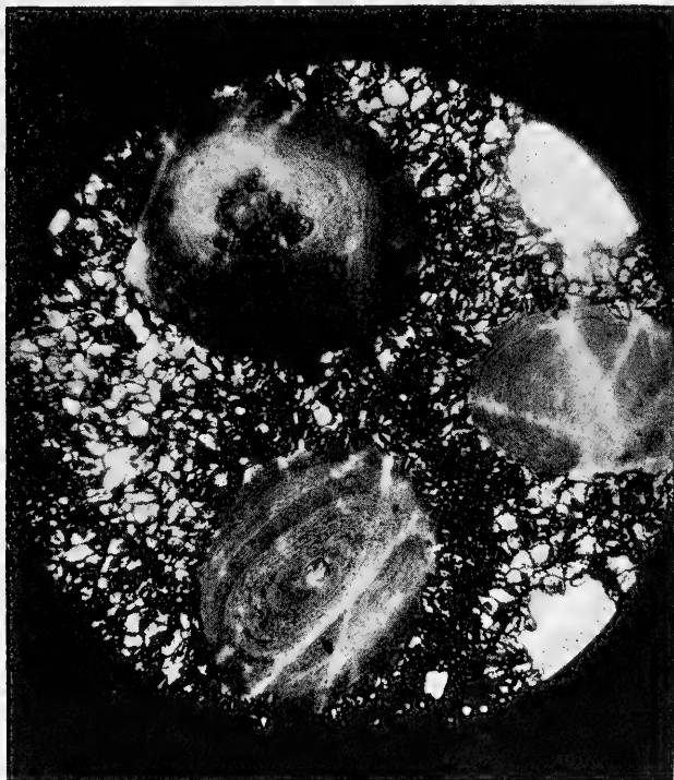
FIG. 1.—Photomicrograph of oölitic grains of a light green silicate in a groundmass of siderite and (secondary) iron hydroxide, forming a local facies of the Onondaga limestone near Preston, Bath County, Kentucky. Note the free edges of the siderite crystals extending into the oölitic grains, cutting through their structure, mostly without disturbing it; also the discordance between outline and structure of the grain near the lower margin. (The longest diameter of this grain measures 0.7 mm.)
