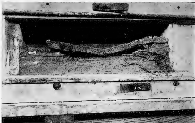
FIG. 11.—Slice faulting, developing an imbricate structure. The bottom layer was composed of pure clay; the next above of mixed sand and clay; the third was a thin layer of sand; and the heavy competent layer at the top was made of plaster two parts, sand one part and clay one part. The brittle top layer arched up and fractured as the first slice fault developed. Each successive slice fault broke out below and in front of its predecessor.
