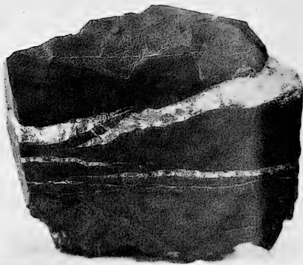
FIG. 4.—Calcite veins in limestone showing inclusions of the wall rock. Two-thirds natural size.
