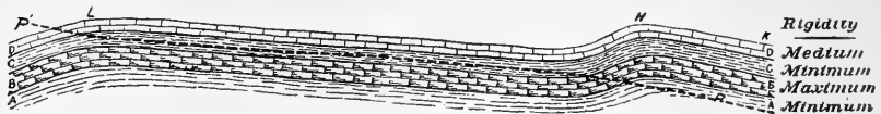
FIG. 2.—A theoretical section to represent the position of the fault plane ( PP' ) in the Rome and Cartersville thrusts. From Hayes.
