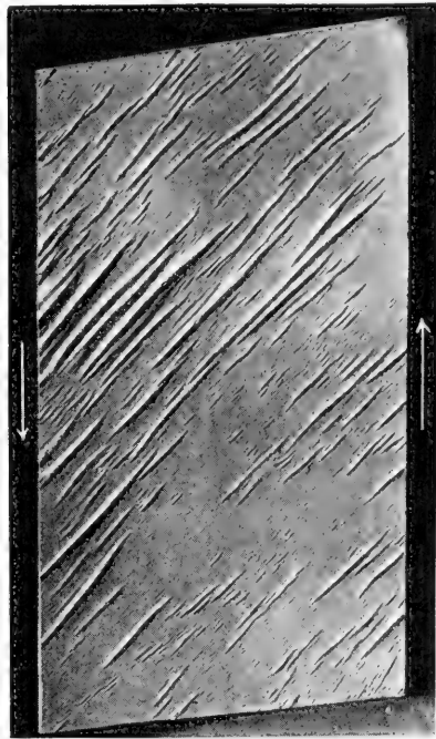
FIG. 12.—Vertical view of reproduction in plaster of Paris of folds produced by shearing deformation. The direction of movement is indicated by arrows and the amount of deformation is shown by the shape of the block.
