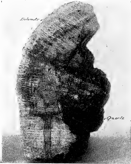
FIG. 1.—Wood replaced by dolomite. Gray part is compact dolomite showing radial lines and small black siliceous dots, which may represent location of resin ducts. In center of specimen is coarser dolomite in rhombs and compound groups. Black portion, showing annual rings, is quartz. (Slightly reduced.)
