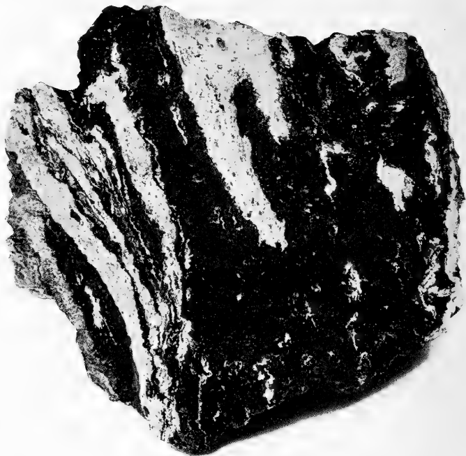
FIG. 11.—Specimen of banded pumice (4×4 inches) from the deposit in the Valley of Ten Thousand Smokes. Adjacent bands show marked differences in composition, as indicated by a silica content of 74.70 per cent in the case of a light band, and 60.40 per cent in an adjacent dark band. The structure is believed to be due to digestion of foreign material.
