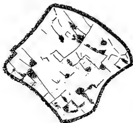
FIG. 1.—Micro-drawing of quartz, multiplied 47 diameters, showing cleavage.
