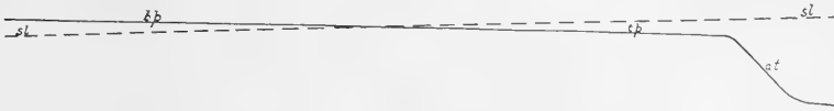
FIG. 2.— b p Continental base-plain. sl Sea level. t p Submerged terrace plain. a t Abysmal terrace face.
