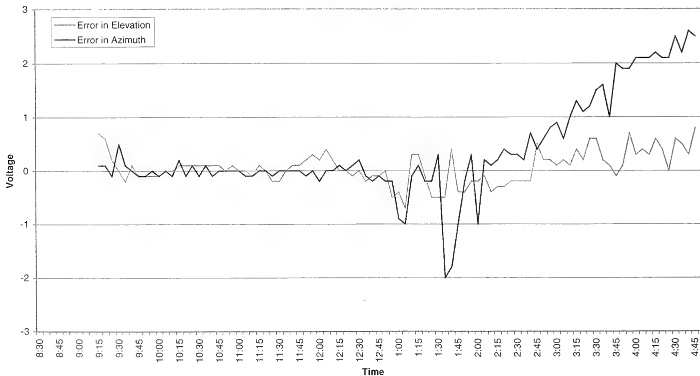
Figure 4. Morehead Radio Telescope, Morehead State University, Morehead, Kentucky. Error of azimuth and elevation as a function of time. These data were taken on 7 Apr 2002.
