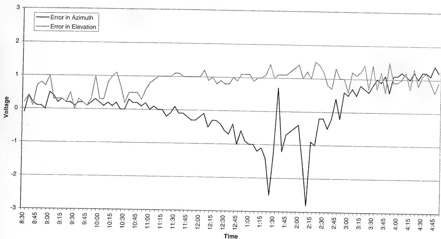
Figure 5. Morehead Radio Telescope, Morehead State University, Morehead, Kentucky. Error of azimuth and elevation as a function of time. These data were taken on 7 April 2002.
