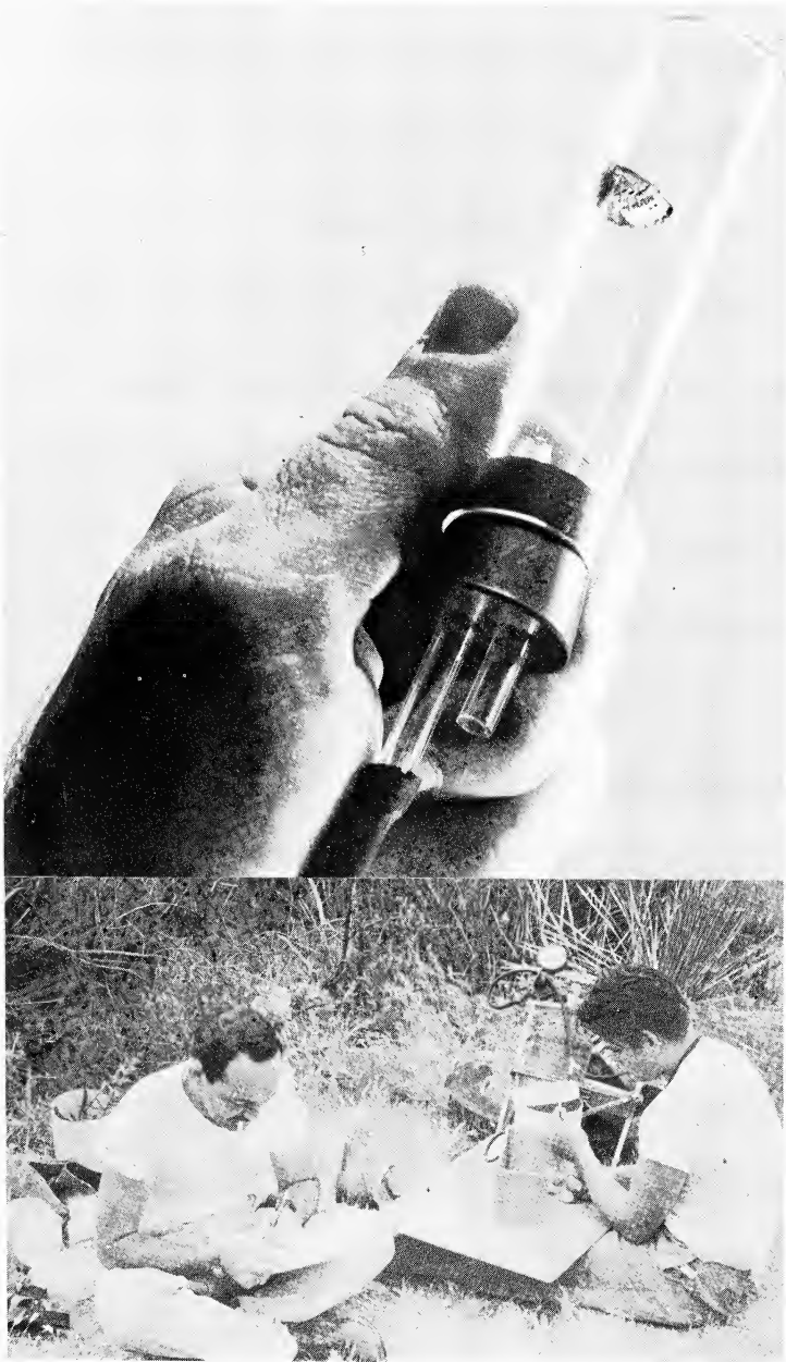
Fig. 2. (below) Photograph showing equipment described in the text. RHTM on right holding a specimen about to be placed in the recovery chamber on the portable desk. Vials with specimens can be seen in the compartment and the CO 2 tank behind. MSRS on left recording data.
